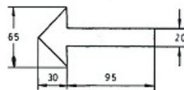
6A For Pipes DN 200 and Below
