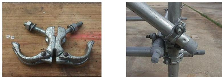
The swivel clamp attaches tubes at various angles. It is used for diagonal braces.
